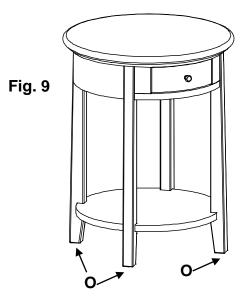
10. Place the table at its final destination. To level the table, rotate the Adjustable Glides (O) found on the bottoms of the legs. See Figure 9.
