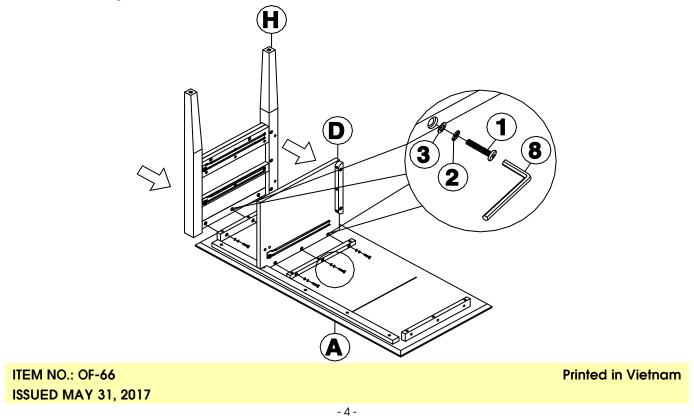
Attach back panel (G) to vertical panel (D) and side frame (H) with bolts (1), and washers (2) and (3) as shown below. Tighten with Allen key (8).
