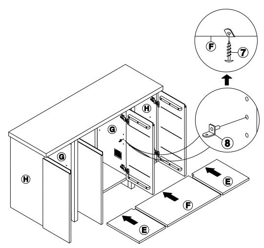
Attach steel bands (10) to the unit with screws (7) as shown below. (to secure the product to the wall and reduce the risk of tipping over).
